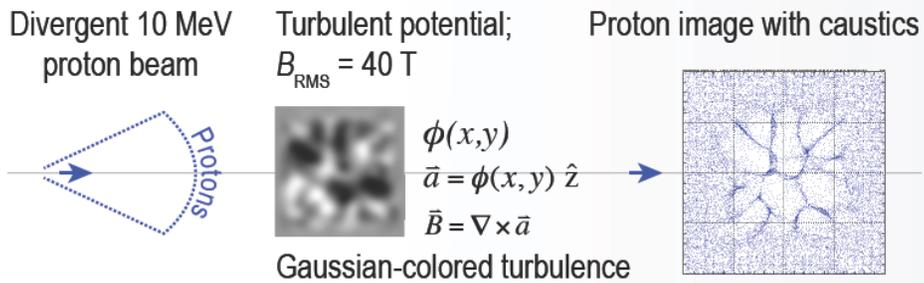
Proton motion was traced using the LSP (PIC) code in 3D. We see that soft turbulent objects generate sharp caustics in the proton image.
